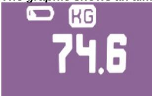
This means that the batteries are almost empty. The scale can still measure weight but no more impedance. To measure impedance again, batteries need to be replaced with new ones. Discard all used batteries and wait at least 30 seconds before inserting the new ones so that the scales have time to restart. If you do not wait long enough you might see the ""low battery"" indicator displayed, and therefore won't be able to get your impedance measurements."
