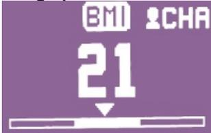
This screen displays the BMI of the user, and represents it with an arrow on a bar, the full part of which falls within recommended values (between 18 and 25). If the user has been recognised, his nickname will be shown in the top right of the screen (CHA on the image).
