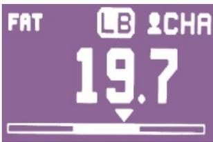
This screen displays the fatty mass of the user, representing it with an arrow on a bar, the full part of which corresponds to the 'normal' zone.
