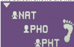
If several people have similar weights, the scale asks the user to confirm the name associated with the current measurement. To do this, move the arrow until it is pointing at your nickname by shifting your weight from one foot to the other (depending on which way you want to move the arrow). Then stand still and wait until your nickname is confirmed.
