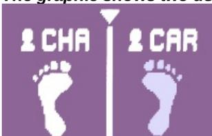
This means that the scale is hesitating between two users with similar weights to assign the measurement. To choose between the two users you just have to step on the side bearing the name of the correct user and raise your other foot."
