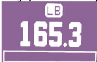
This means that the impedance measurement is about to begin. If the loading bar stays empty and does not flash, this means that impedance measurement was not possible because the user is not barefoot. In this case, only weight is recorded."
