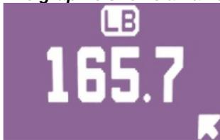
This means that the user is positioned too far to the right and rear of the scales and should reposition himself more in the centre. Likewise an arrow in the top right of the screen means that the user is too far to the right and front of the scales."
